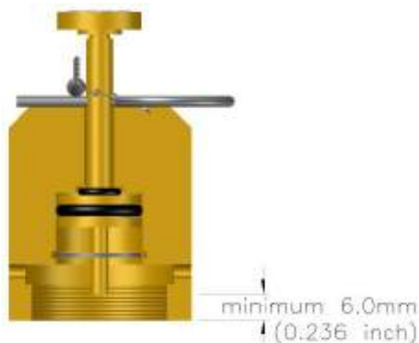
Figure 43 Manual Actuator in Non-Fire Position
