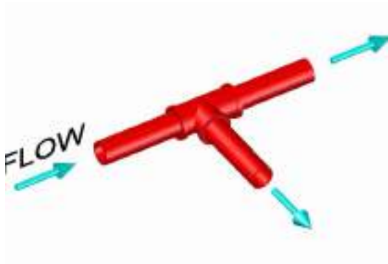
Figure 29 Correct Side Tee Splits Orientation
