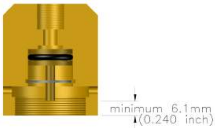
Figure 45 Pneumatic Actuator in Non-Fire Position
