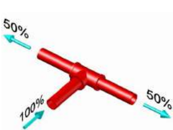
Figure 24 Minimum Bull Tee Imbalance
