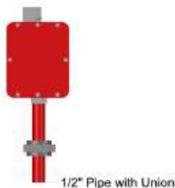
Figure 54: Distribution pipe / Manifold- Discharge Pressure Switch Installation
