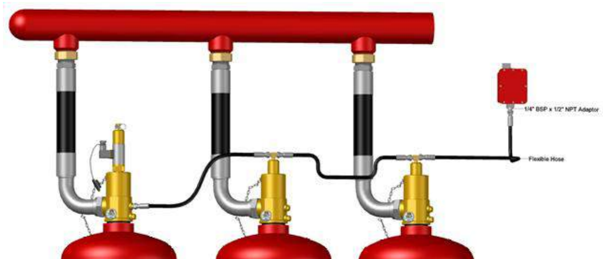
Figure 53: Multiple Cylinder System - Discharge Pressure Switch Installation
