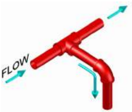
Figure 29 Correct Side Tee Splits Orientation
