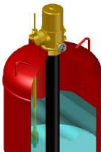
Figure 21 Liquid level indicator
