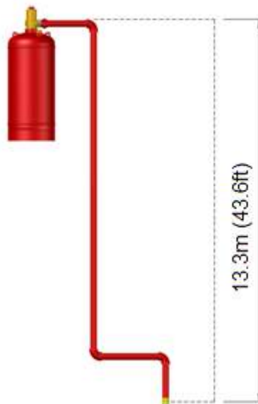
Figure 35 Nozzles Located Below the Cylinder Outlet
