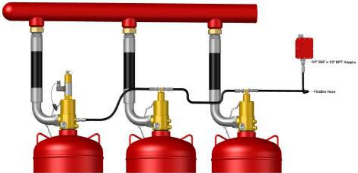
Figure 53: Multiple Cylinder System - Discharge Pressure Switch Installation
