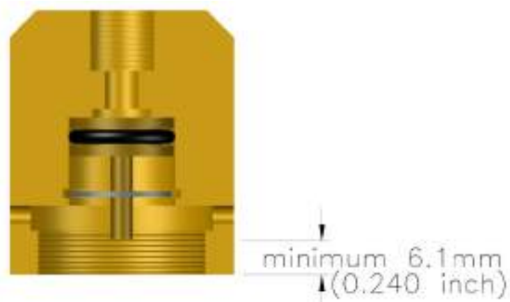
Figure 45 Pneumatic Actuator in Non-Fire Position
