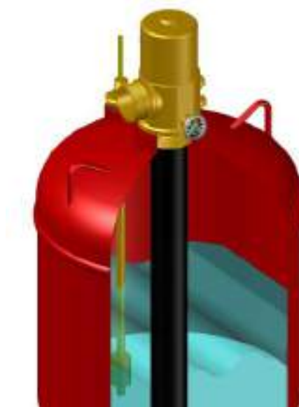
Figure 22 Liquid level indicator
