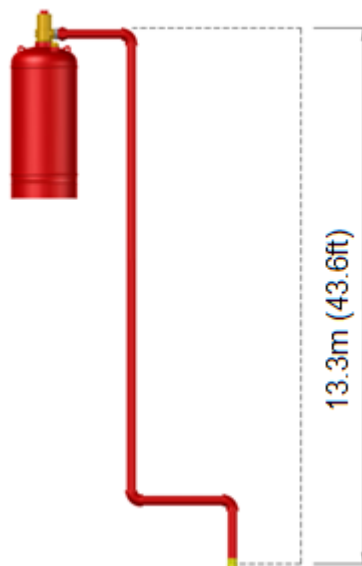
Figure 35 Nozzles Located Below the Cylinder Outlet
