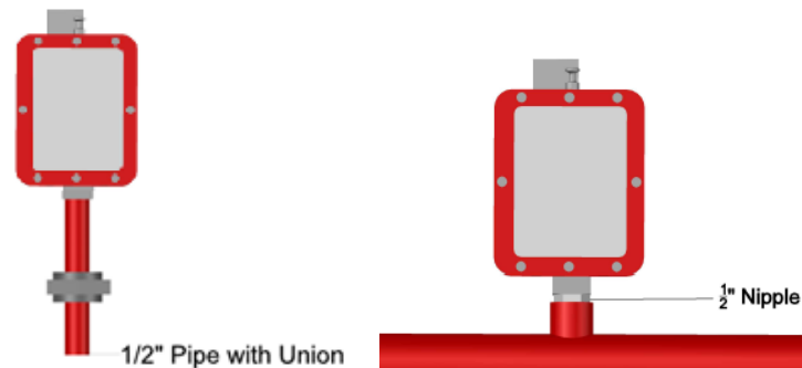
Figure 4.5.2: Distribution pipe / Manifold- Discharge Pressure Switch Installation
