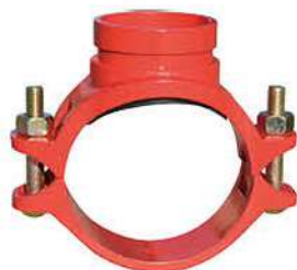
Style 3G Grooved Outlet Mechanical Tee DN65X25~DN200X100 2X1 1/8X4" 60.3X33.7mm~219.1X114.3mm
