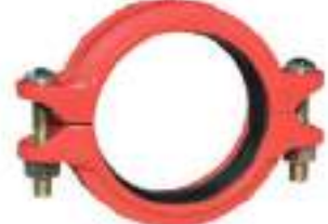
Style 1GS Rigid Coupling 300 PSI • UL + FM 1–12 in
