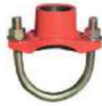
Style 3L U-bolt Mechanical Tee 1¼" × ½" ~ 2½" × 1" 200 psi most sizes; 300 psi only 1 × ½ in
