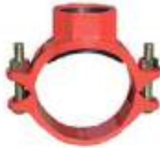
Style 3J Threaded Outlet Mechanical Tee 2½" × ½" ~ 8" × 3" UL + FM: 300 PSI
